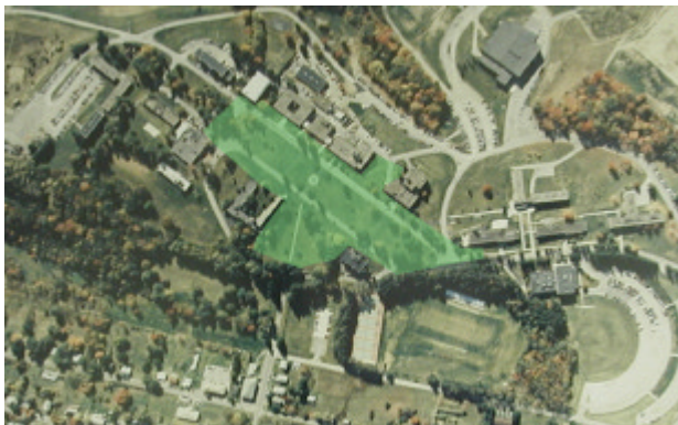
Figure 8: Coverage Pattern of Directional Antenna Facing the Pine Bowl on Schwab Hall
