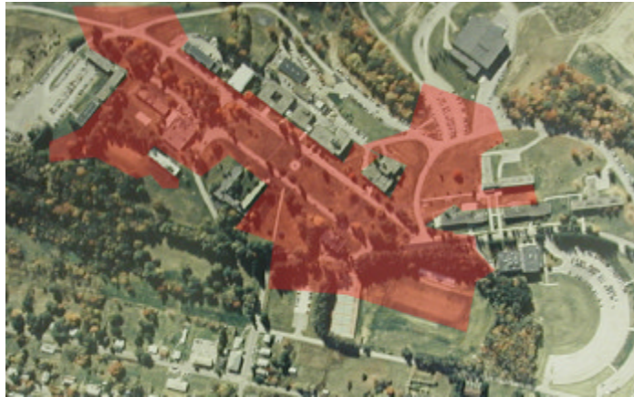
Figure 11: Composite Coverage Area of all Antennas
